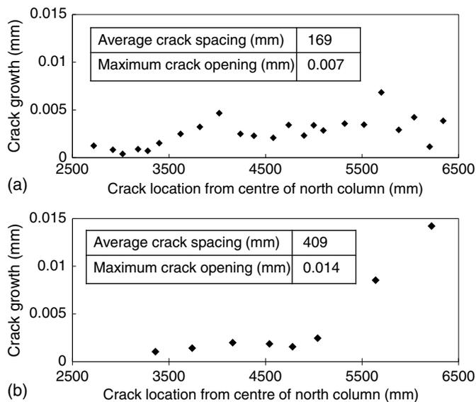
**Fig. 6.** Cracking behavior due to six scissor lifts at bottom fiber height: (a) beam; and (b) drop.
