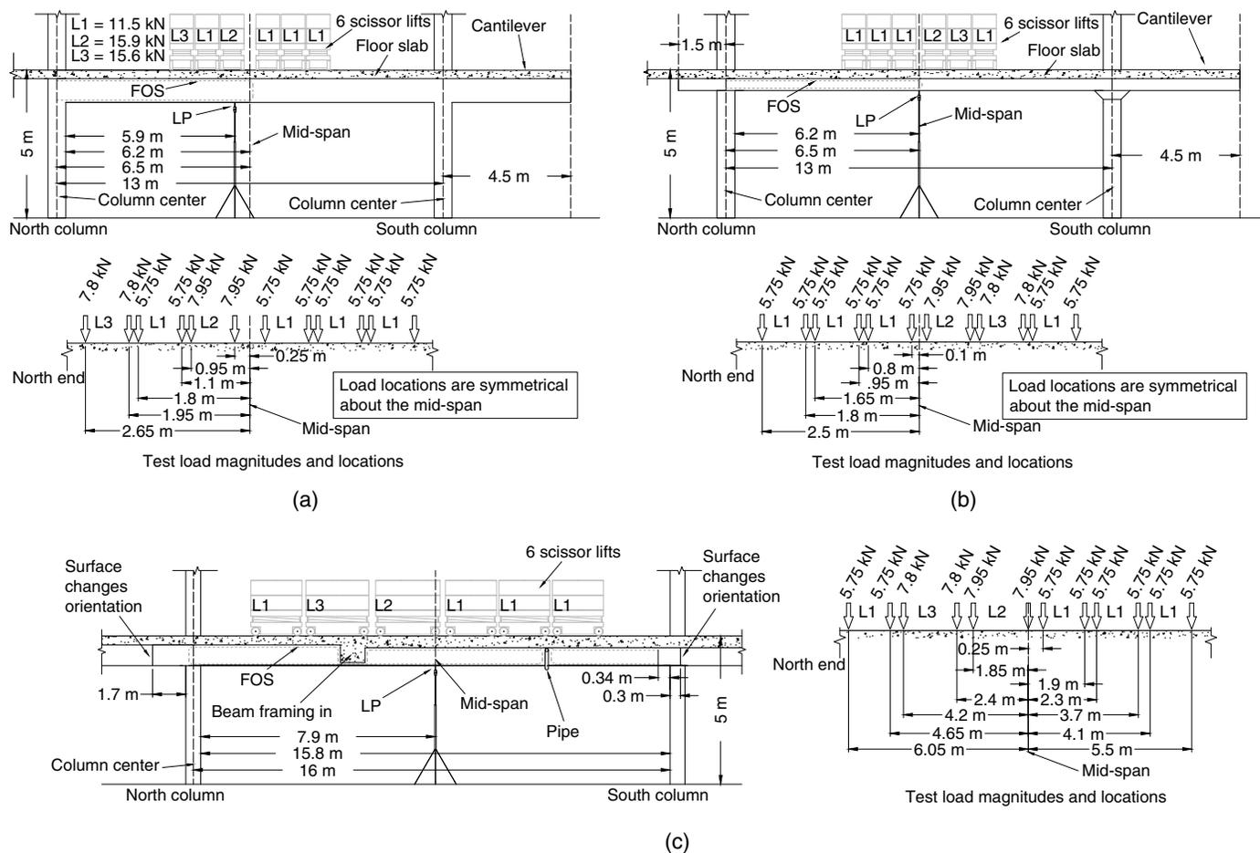
Fig. 4. Elevation view of the load test setups: (a) beam; (b) drop; and (c) large beam.
