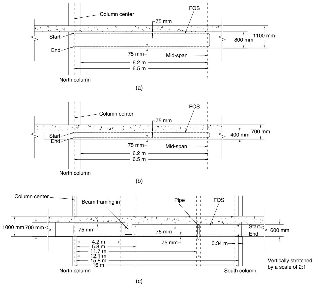
Fig. 2. Elevation view of the FOS instrumentation: (a) beam; (b) drop; and (c) large beam.
