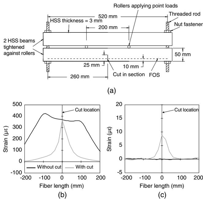
**Fig. 9.** Aluminum test apparatus: (a) apparatus schematic; (b) FOS strain measurements when loaded; and (c) FOS strain measurements when unloaded.
