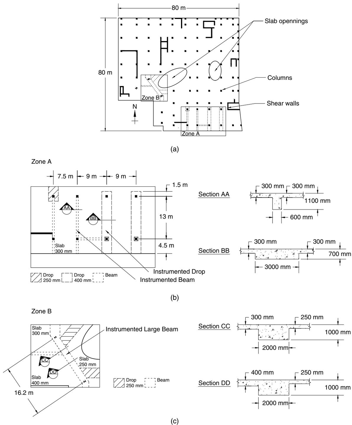
**Fig. 1.** Plan view of Level 4: (a) full level including Zone A and Zone B; (b) Zone A including the beam and drop; and (c) Zone B including the large beam.
