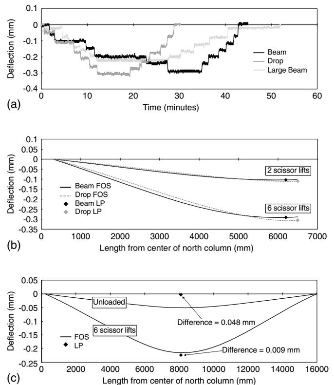
**Fig. 7.** Deflection behavior: (a) full load test LP measurements; (b) beam and drop deflected shape comparison; and (c) large beam deflected shape.
