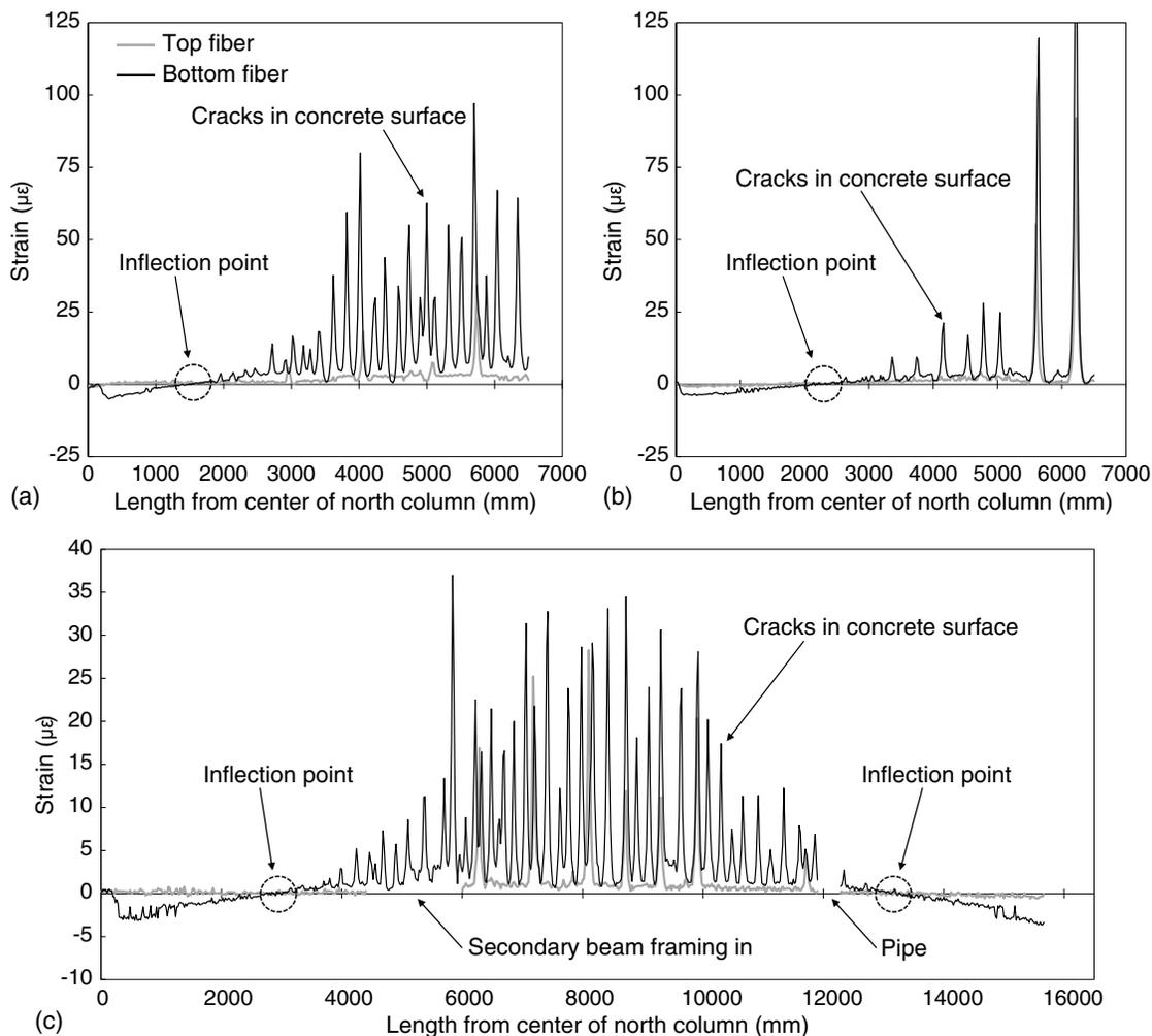
Fig. 5. FOS strains due to six scissor lifts: (a) beam; (b) drop; and (c) large beam.
