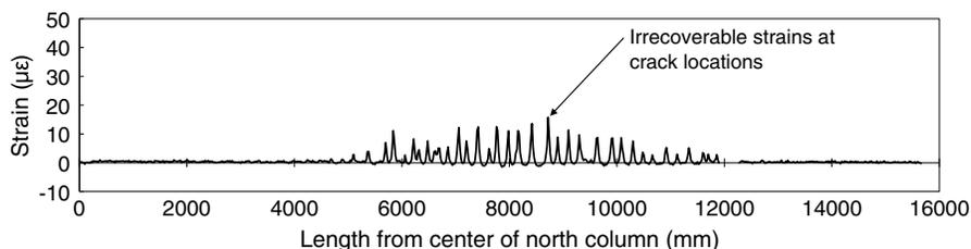
Fig. 8. Bottom fiber strain measurements for the large beam once unloaded.
